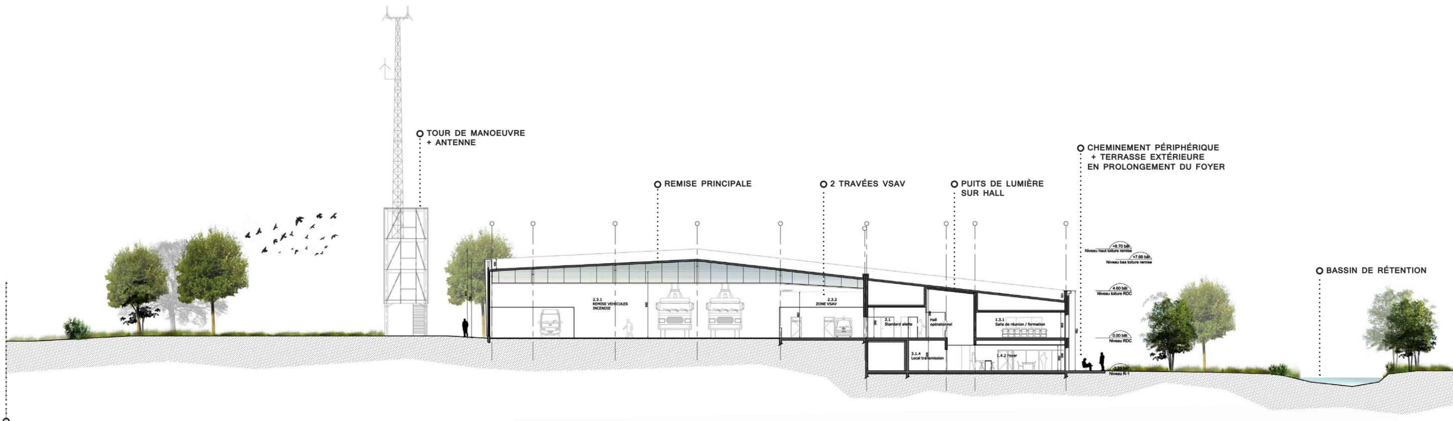
Architectural cross-section diagram showing building layout, levels, and structural elements. The diagram includes a control tower, a main garage, two VSAV bays, a meeting room, and a retention basin. Elevation markers indicate levels such as +8.70 bit, +7.90 bit, +4.50 bit, and +0.00 bit.
